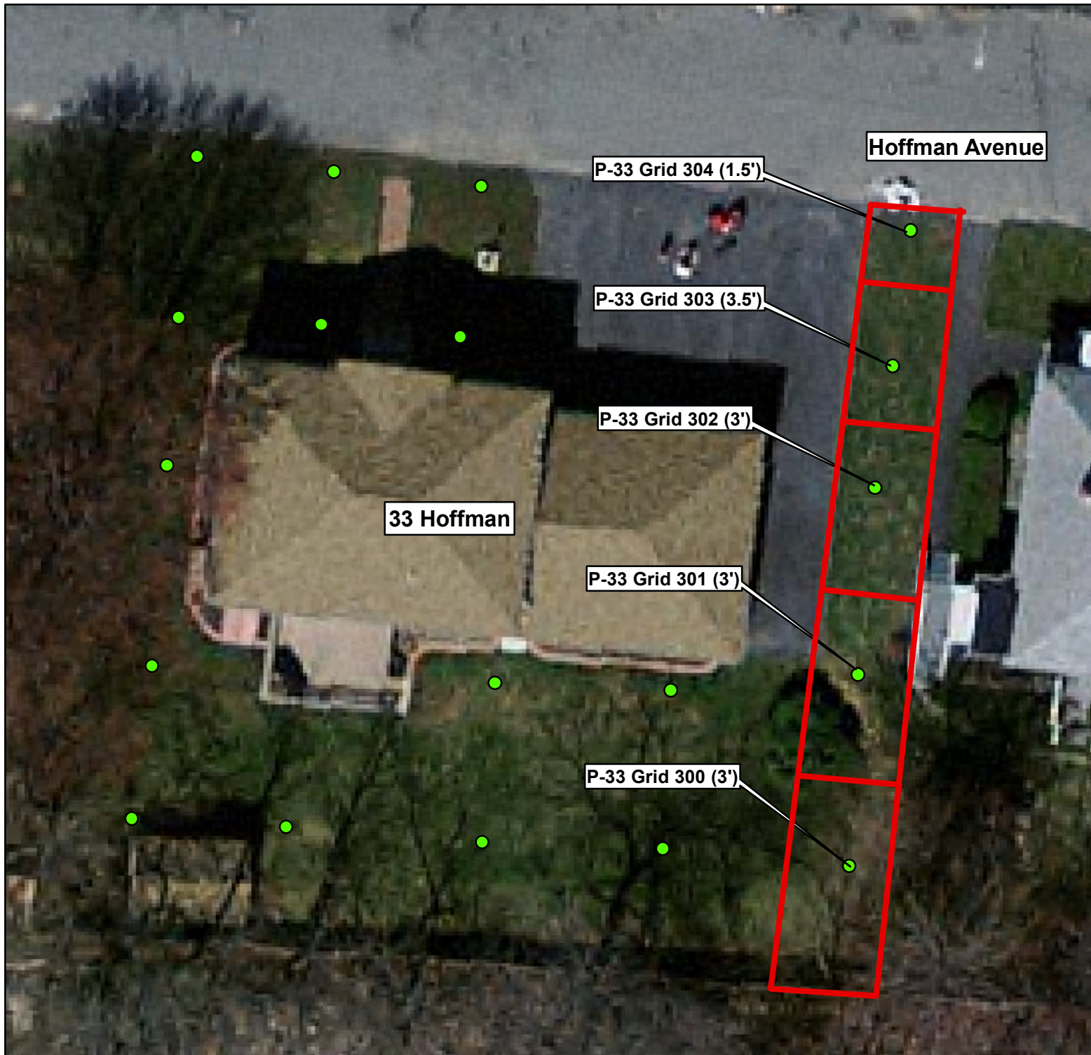
Figure 3 Removal Grid Location Map 33 Hoffman Avenue Tombarello Site 207 Marston Street Lawrence, Massachusetts
