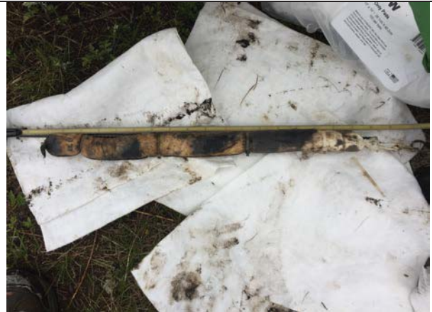
Photo 8: MW-407 – sock removed 6 days after installation, 4/25/17.
