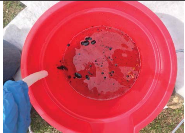
Photo 2: MW-201 – NAPL and water discharge, 4/17/17.
