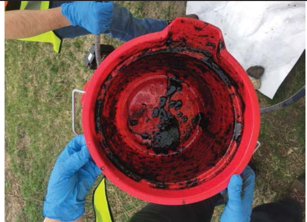
Photo 4: MW-201 – NAPL adhered to inside of pail, 4/17/17.
