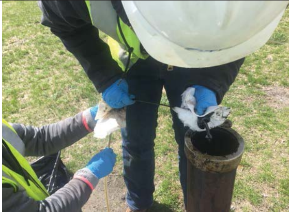
Photo 7: MW-414 – NAPL being removed from tape, 4/18/17.
