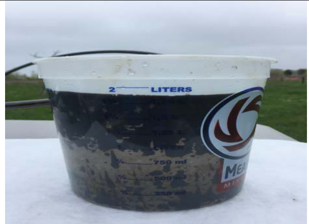
Photo 14: MW-414 – NAPL and water discharge side, 5/1/17.
