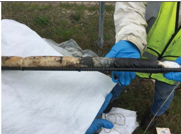
Photo 5: MW-406 – sock removed 6 days after installation, 4/25/17.
