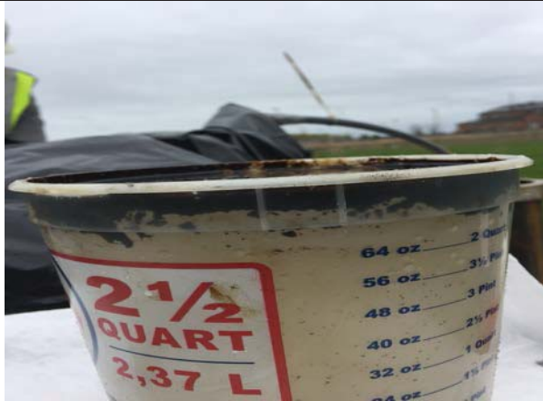
Photo 13: MW-414 – NAPL and water side view, 4/25/17.
