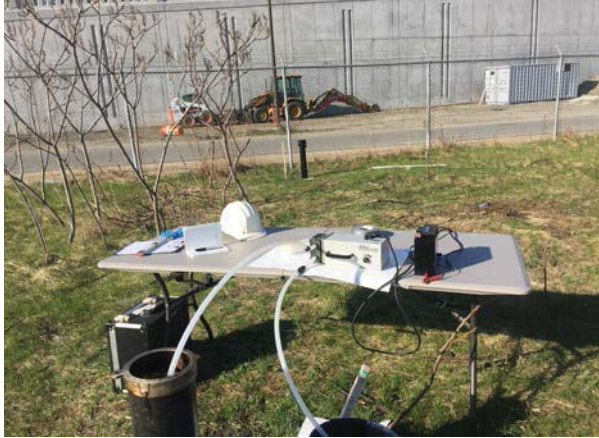
Photo 1: MW-414 – skimming test setup, 4/17/17.
