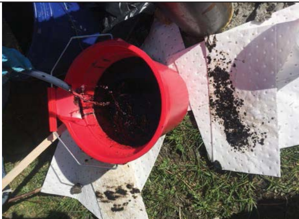
Photo 3: MW-414 – NAPL and water discharge, 4/17/17.
