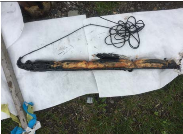
Photo 3: MW-201 – sock removed 6 days after installation, 5/1/17.
