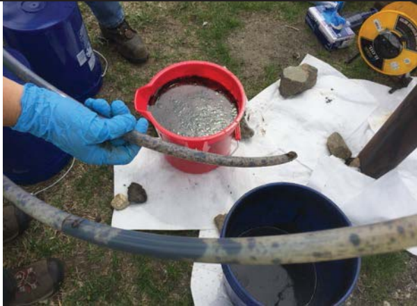
Photo 3: MW-201 – NAPL in tubing and floating in pail, 4/17/17.
