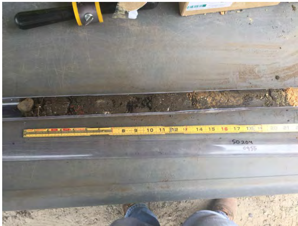
SCENE: View of top section (0 to 2 feet) of soil boring SB-204.
