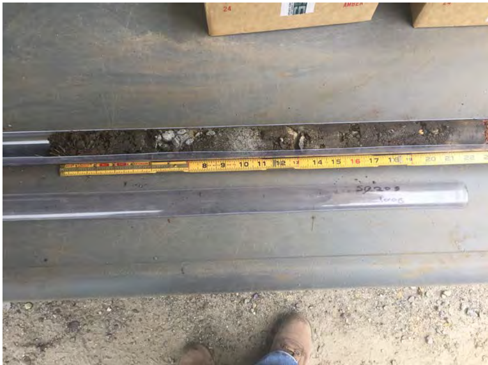
SCENE: View of top section (0 to 2 feet) of soil boring SB-205.
