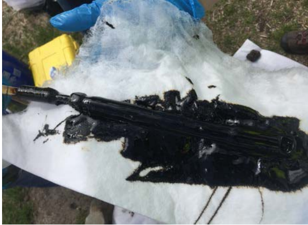
Photo 1: MW-201 – NAPL coating probe and pad, 4/17/17.
