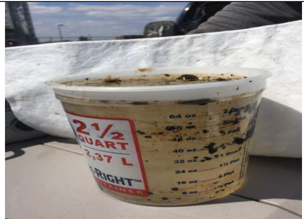
Photo 10: MW-414 – water and NAPL globs – side view, 4/19/17.
