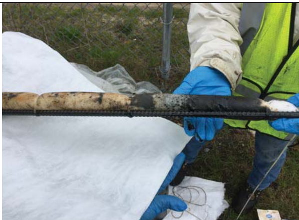
Photo 5: MW-406 – sock removed 6 days after installation, 4/25/17.
