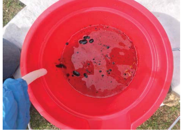
Photo 2: MW-201 – NAPL and water discharge, 4/17/17.
