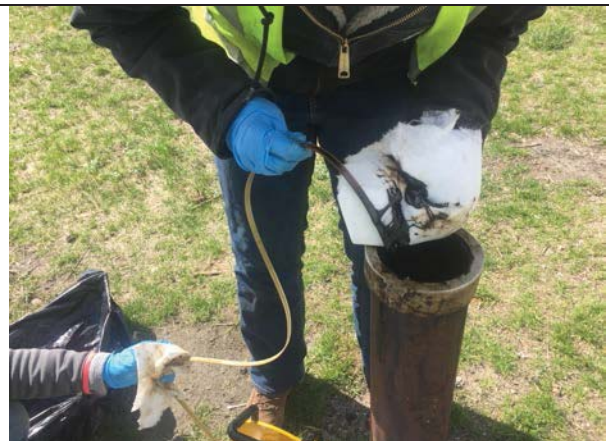
Photo 6: MW-414 – NAPL coating tape, 4/18/17.
