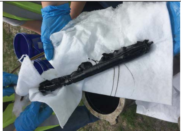
Photo 4: MW-414 – NAPL coating probe, 4/17/17.
