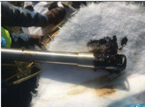
Photo 5: MW-414 – water and NAPL on probe tip, 4/18/17.
