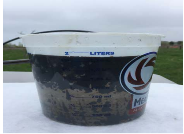
Photo 14: MW-414 – NAPL and water discharge side, 5/1/17.
