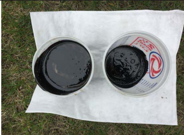
Photo 15: MW-414 – NAPL and water discharge into left container, and partial decant to right container, 5/1/17.
