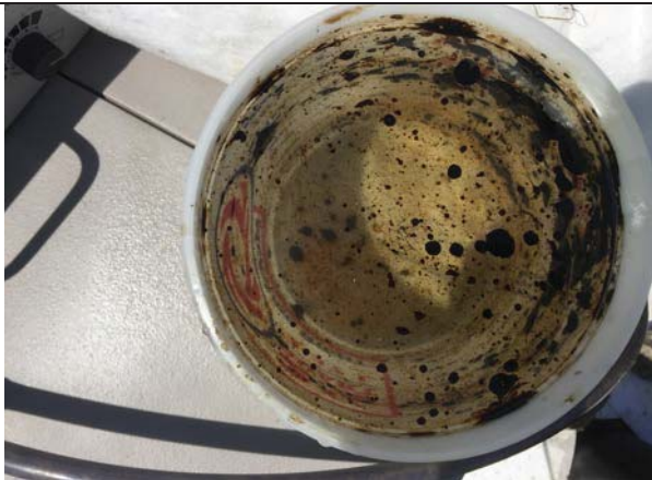
Photo 9: MW-414 – water and NAPL globs – top view, 4/19/17.
