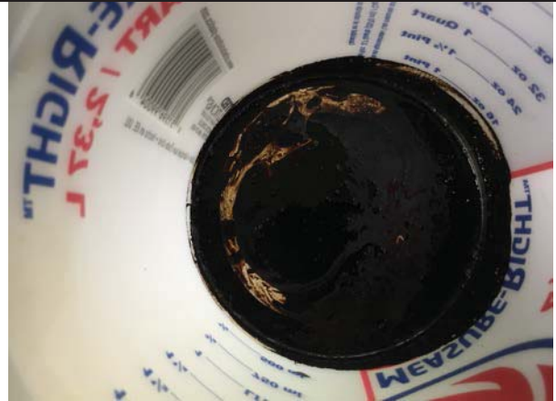
Photo 16: MW-414 – NAPL and water decanted top, 5/1/17.
