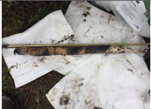
Photo 8: MW-407 – sock removed 6 days after installation, 4/25/17.
