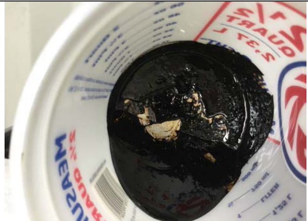
Photo 18: MW-414 – NAPL and water, most water decanted off, 5/1/17.
