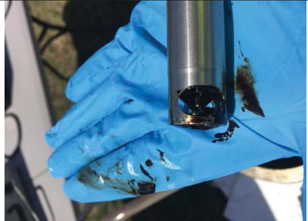
Photo 8: MW-414 – NAPL and water on probe tip, 4/19/17.
