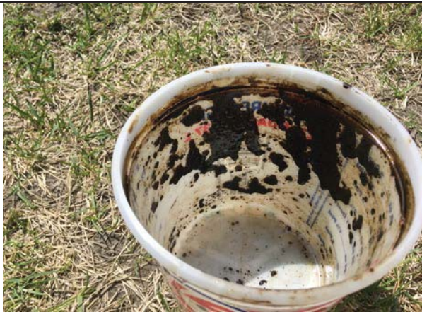
Photo 11: MW-414 – NAPL coating 2.5 quart container-side, 4/19/17.
