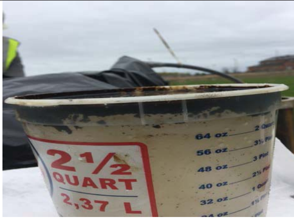
Photo 13: MW-414 – NAPL and water side view, 4/25/17.
