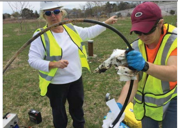
Photo 6: MW-201 – NAPL plugging ½-inch inside diameter peristaltic tubing on 4/17/17.
