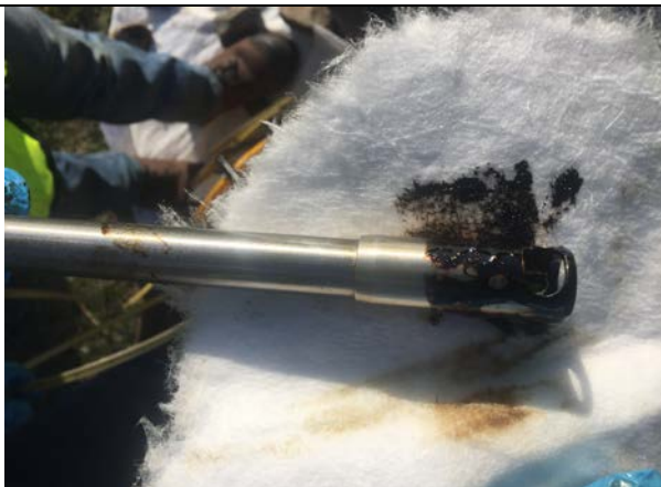
Photo 5: MW-414 – water and NAPL on probe tip, 4/18/17.
