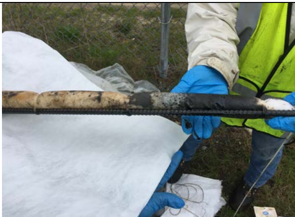
Photo 5: MW-406 – sock removed 6 days after installation, 4/25/17.
