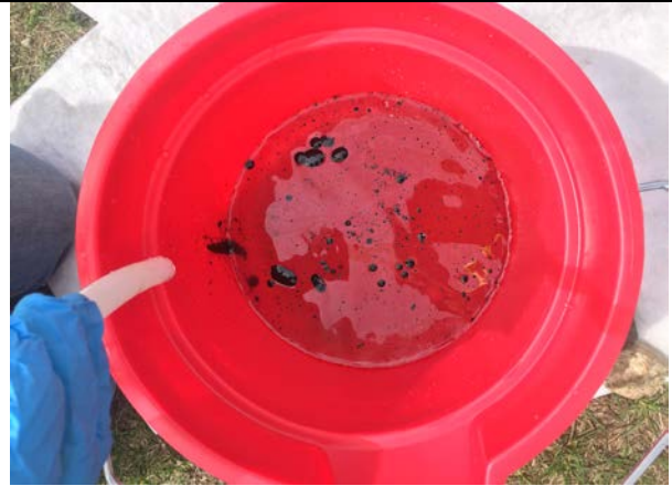
Photo 2: MW-201 – NAPL and water discharge, 4/17/17.
