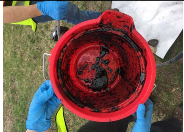
Photo 4: MW-201 – NAPL adhered to inside of pail, 4/17/17.
