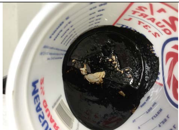
Photo 18: MW-414 – NAPL and water, most water decanted off, 5/1/17.
