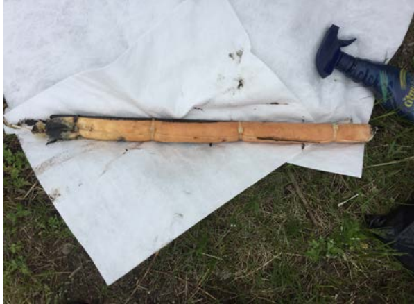
Photo 9: MW-407 – sock removed 6 days after installation, 5/1/17.
