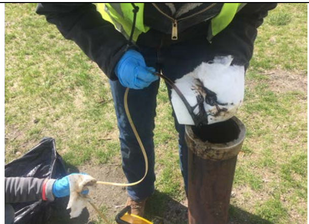
Photo 6: MW-414 – NAPL coating tape, 4/18/17.
