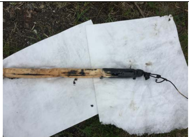
Photo 6: MW-406 – sock removed 6 days after installation, 5/1/17.
