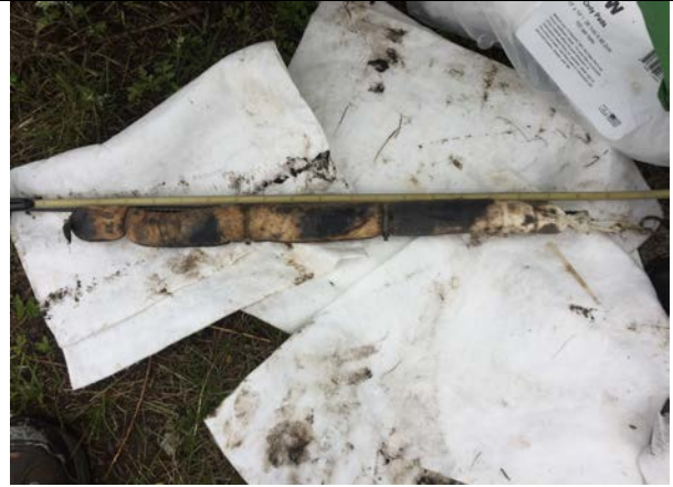
Photo 8: MW-407 – sock removed 6 days after installation, 4/25/17.
