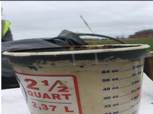
Photo 13: MW-414 – NAPL and water side view, 4/25/17.
