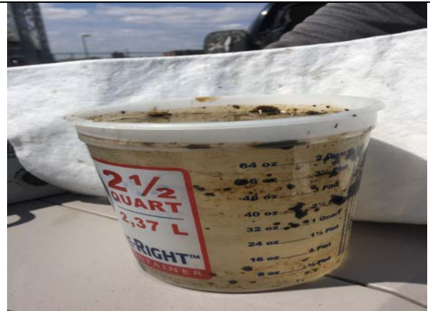
Photo 10: MW-414 – water and NAPL globs – side view, 4/19/17.
