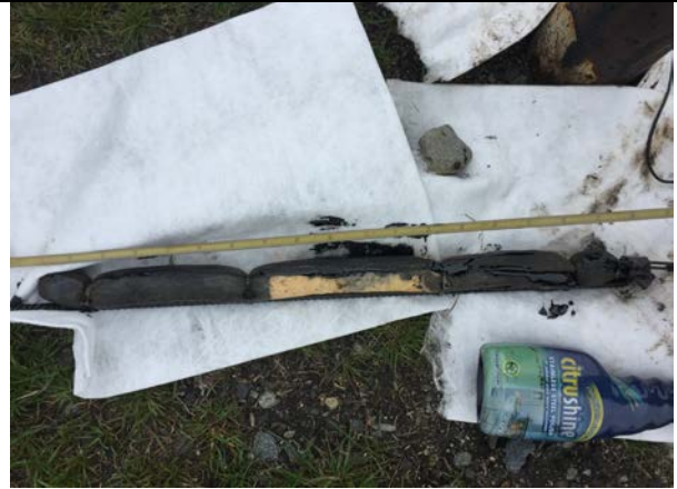
Photo 2: MW-201 – sock removed 6 days after installation, 4/25/17.
