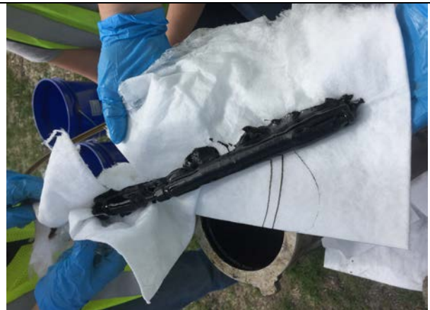
Photo 4: MW-414 – NAPL coating probe, 4/17/17.
