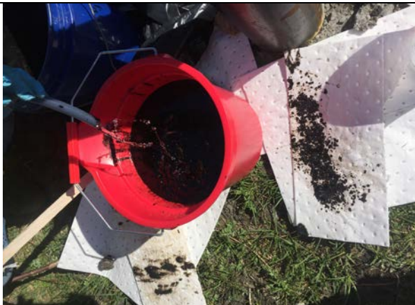
Photo 3: MW-414 – NAPL and water discharge, 4/17/17.
