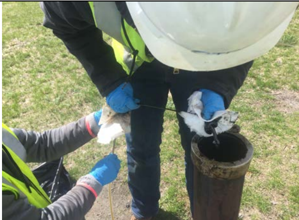
Photo 7: MW-414 – NAPL being removed from tape, 4/18/17.
