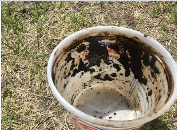
Photo 11: MW-414 – NAPL coating 2.5 quart container-side, 4/19/17.
