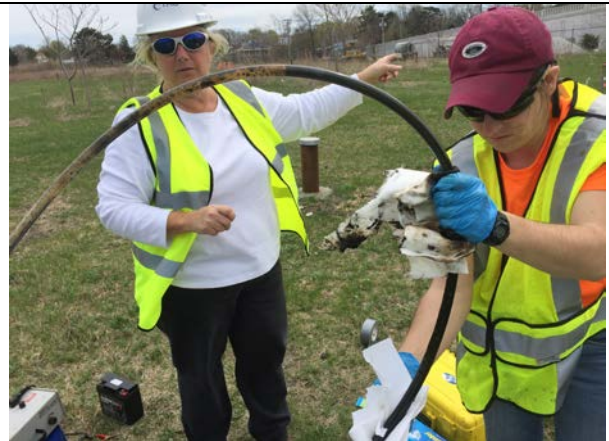
Photo 6: MW-201 – NAPL plugging ½-inch inside diameter peristaltic tubing on 4/17/17.
