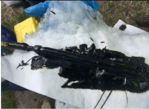
Photo 1: MW-201 – NAPL coating probe and pad, 4/17/17.
