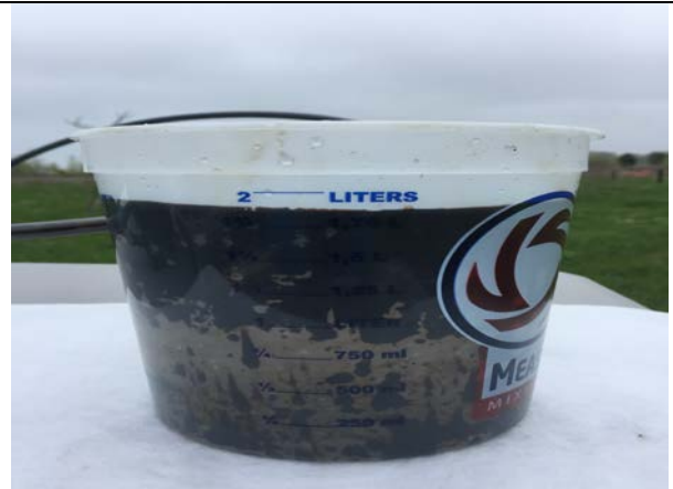
Photo 14: MW-414 – NAPL and water discharge side, 5/1/17.
