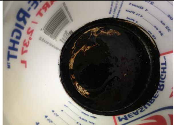
Photo 16: MW-414 – NAPL and water decanted top, 5/1/17.
