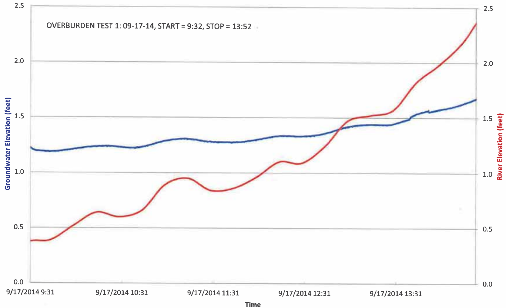
Figure B-30 MW-6 Pumping Test Groundwater Elevation and River Elevation over Time in MW-10D
