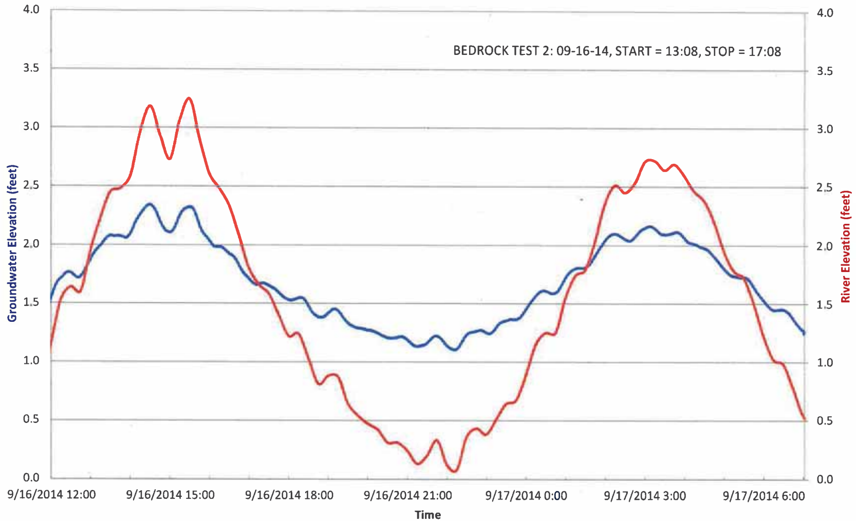
Figure J-19 MW-6B Pumping Test Groundwater Elevation and River Elevation over Time in MW-17B
