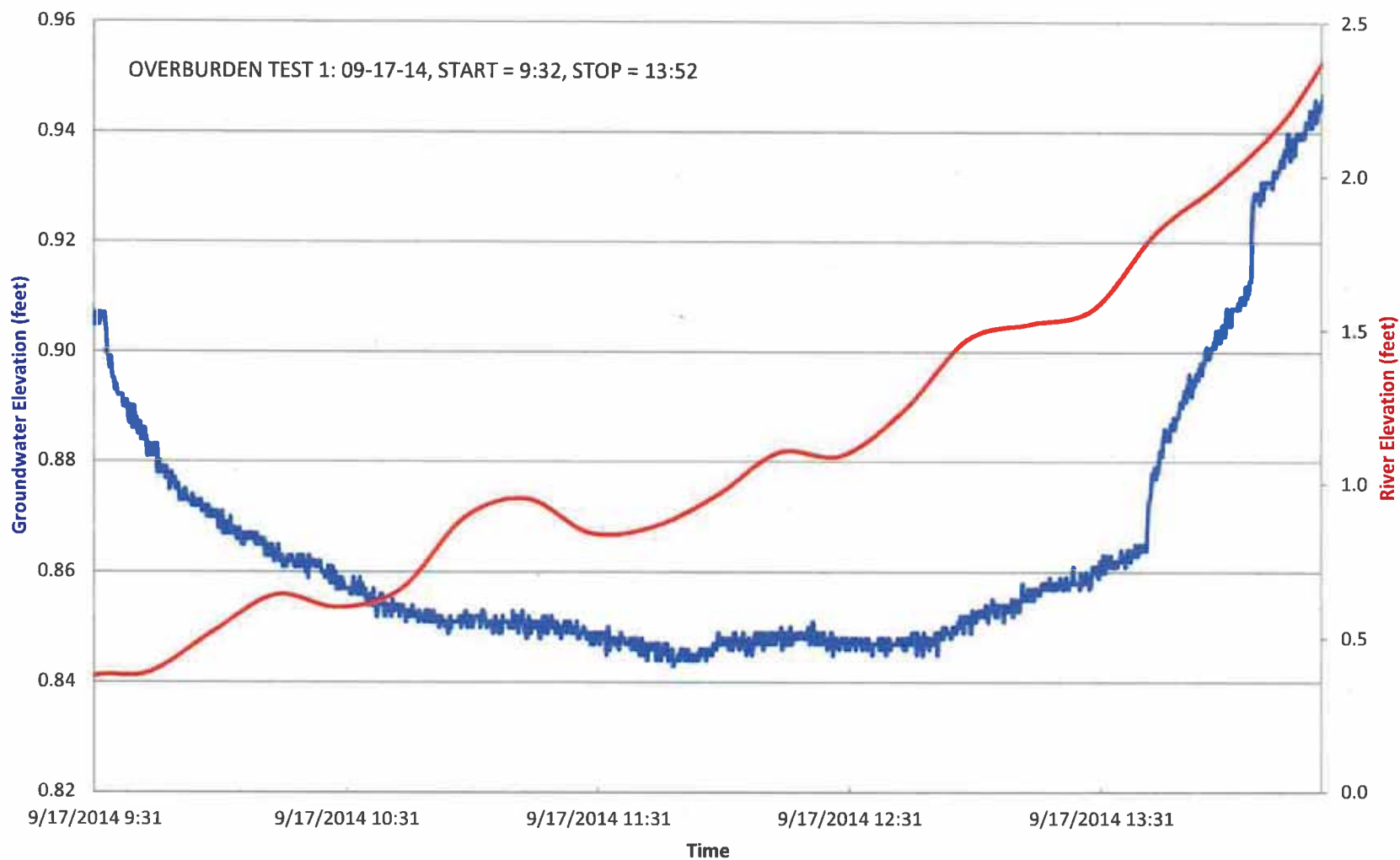
Figure B-41B MW-6 Pumping Test Groundwater Elevation and River Elevation over Time in GZ-102S
