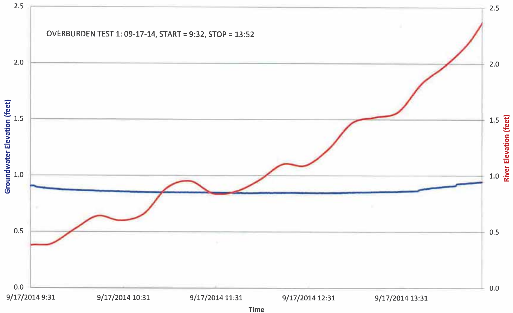
Figure B-41A MW-6 Pumping Test Groundwater Elevation and River Elevation over Time in GZ-102S
