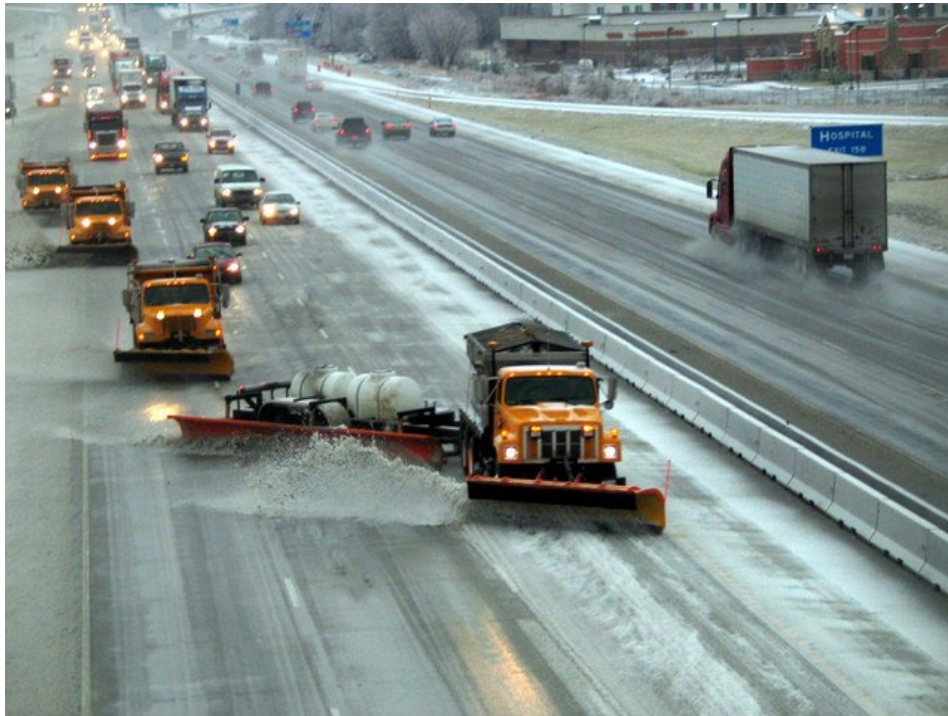
Snowplow Peloton with Tow Plow in Use (Source: MassDOT)
