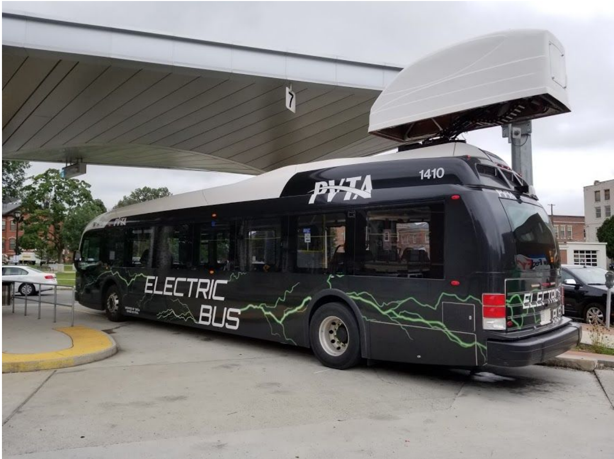
PVTA Electric Bus Charger at Downtown Holyoke Bus Station (Robert Kearns)
