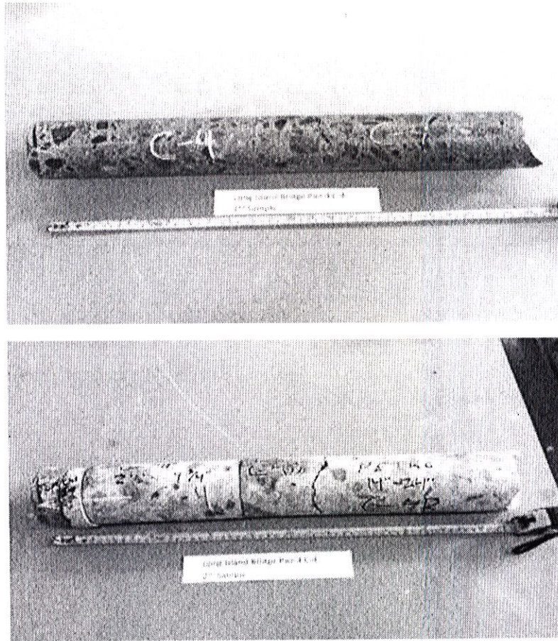
Figure 15 Two C4 cores. An unidentified portion of the top core picture was sent to American Engineering on March 2, 2018 for petro analysis) and the right portion of the bottom picture, the furthest portion from the surface, was sent March 26, 2018). Note: that both are identified as being the 2 nd sample (in error?)
