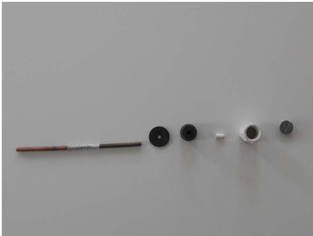
Sample Soil Gas Probe Assembly – Exploded View
