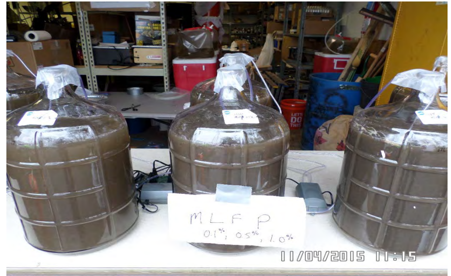
3 MLFP-BP Sediment Slurries (1.0%, 0.5%, and 0.1% solids).
