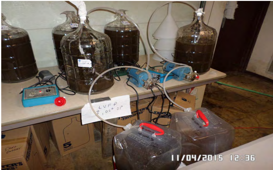
Pumping off LUFBP-BP supernatants after one hour settling. (View 2 of 2)
