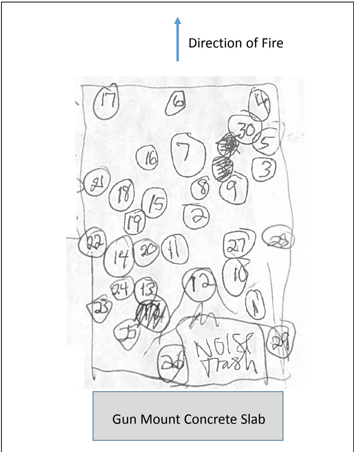
Figure 3-4. Field Sketch Showing Sample Increment Locations at the Near-Range Firing Position and the Areas Where Metallic Debris Prevented Sampling
