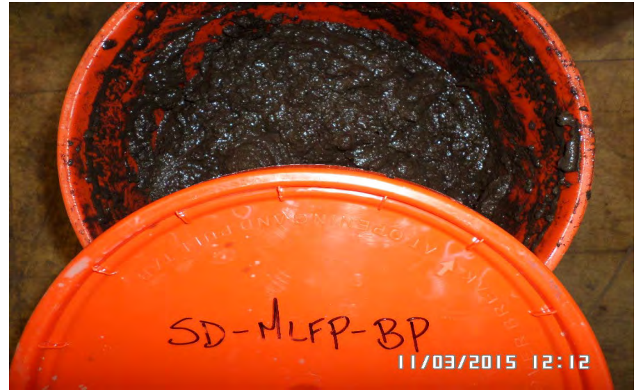
MLFP-BP Sediment after light homogenization.
