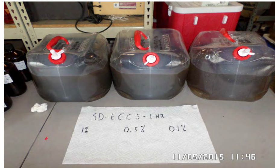
3 ECCS –BP Sediment Slurries (1.0%, 0.5%, and 0.1% solids) during 1 hour aeration stage.
