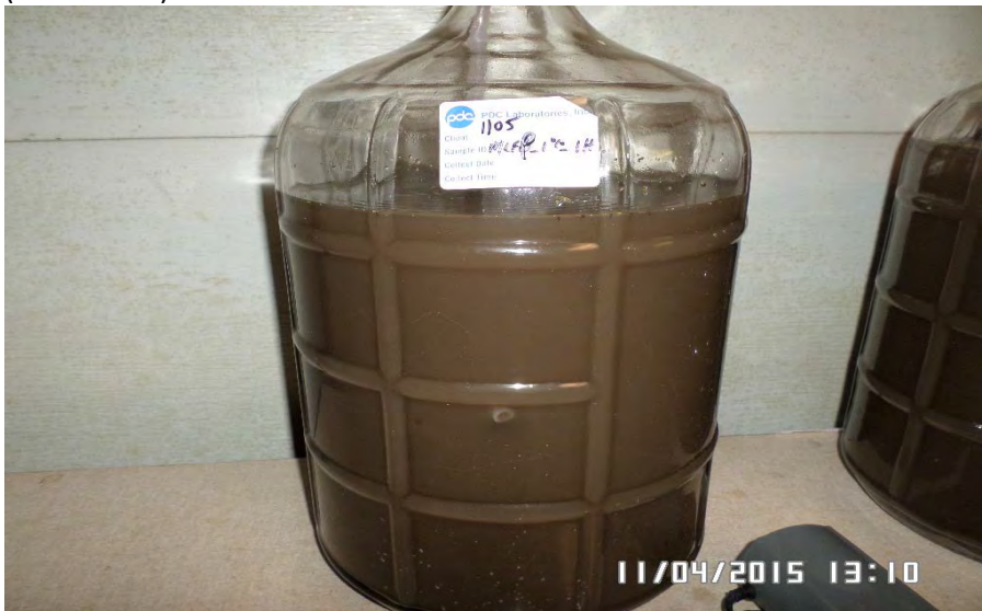
MLFP-BP Sediment Slurry (1 hour aeration at 1.0% solids) after one hour settling.
