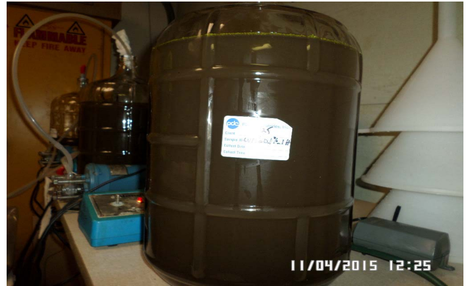
LUFP-BP Sediment Slurry (1 hour aeration at 0.1% solids) after one hour settling.
