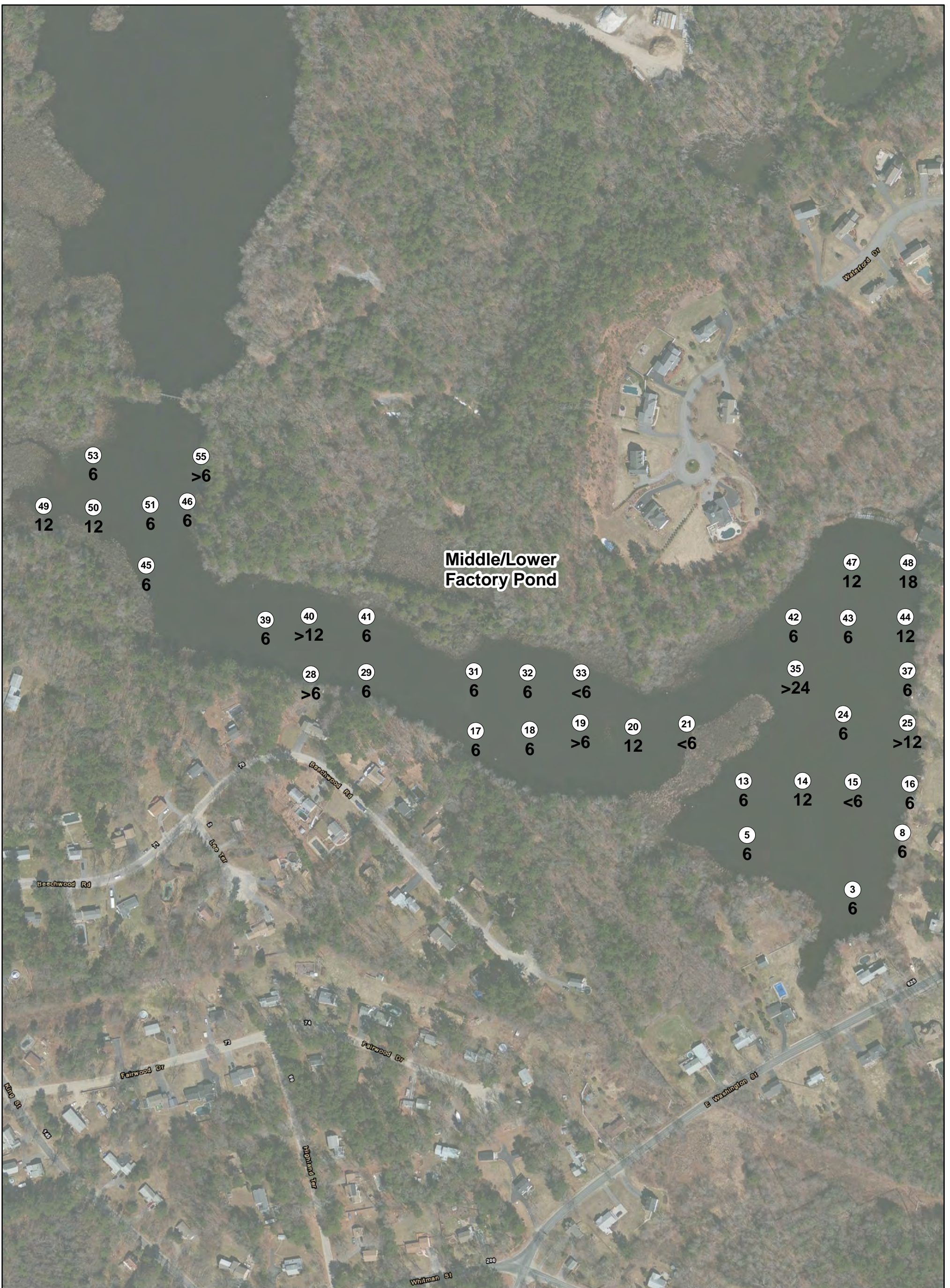
Figure 3-11: Shallowest Depth at Which the Mercury Concentration in Sediment is Less Than 4 mg/Kg
