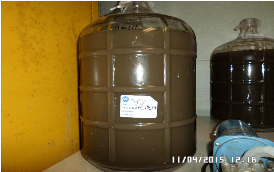
LUFP-BP Sediment Slurry (1 hour aeration at 1.0% solids) after one hour settling.
