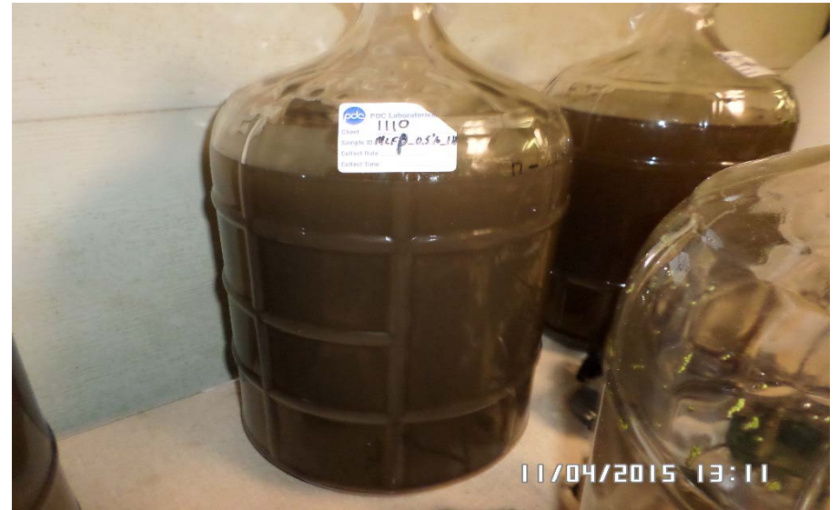
MLFP-BP Sediment Slurry (1 hour aeration at 0.5% solids) after one hour settling.
