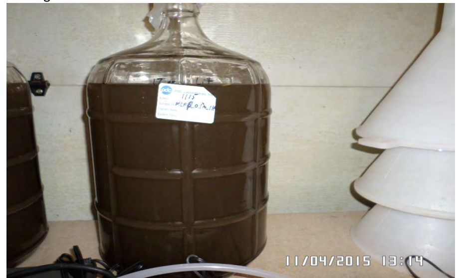
MLFP-BP Sediment Slurry (1 hour aeration at 0.1% solids) after one hour settling.
