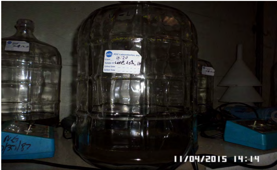
LUF2-BP Sediment after pumping off supernatant (1 hour aeration at 0.5% solids).
