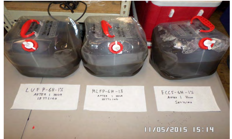
LUFP-BP, MLFP-BP, and ECCS-BP (6 hour aeration at 1.0% solids) supernatants after one hour settling.
