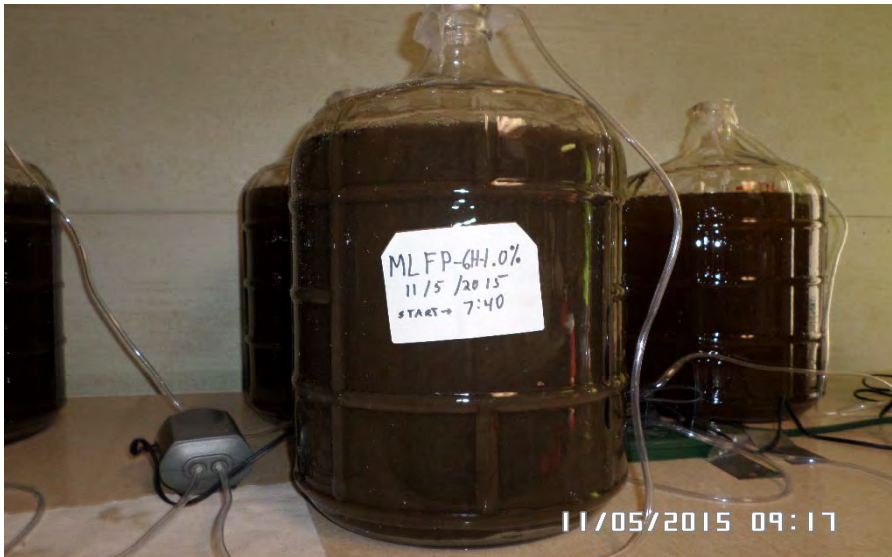
MLFP-BP Sediment Slurry (6 hour aeration at 1.0% solids) during aeration stage.
