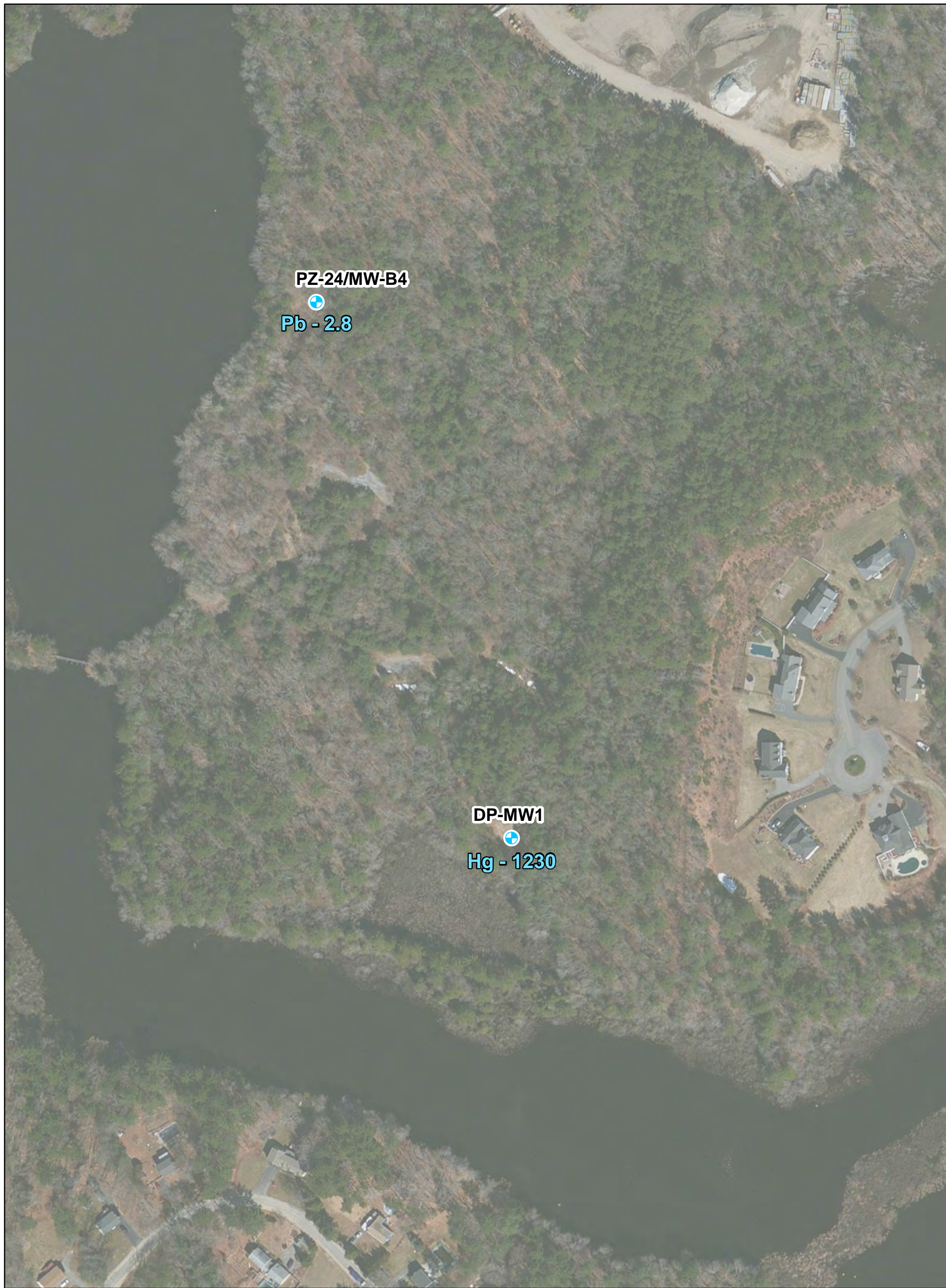
Figure 3-13: Lead and Mercury Concentrations in the Groundwater at Locations Previously Exhibiting Groundwater UCL Exceedances
