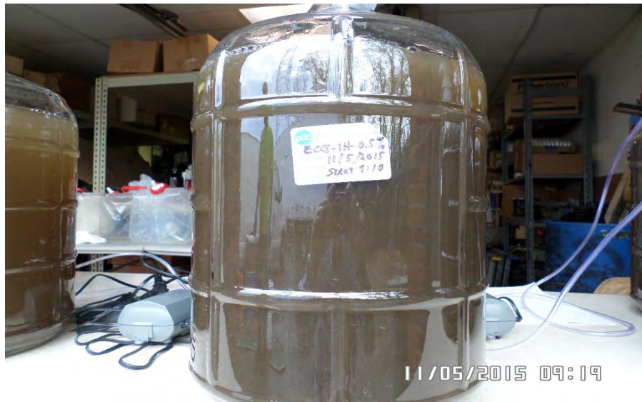
ECCS-BP Sediment Slurry (1 hour aeration at 0.5% solids) during aeration stage.
