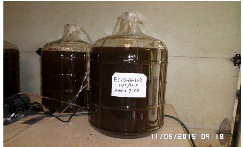
ECCS-BP Sediment Slurry (6 hour aeration at 1.0% solids) during aeration stage.
