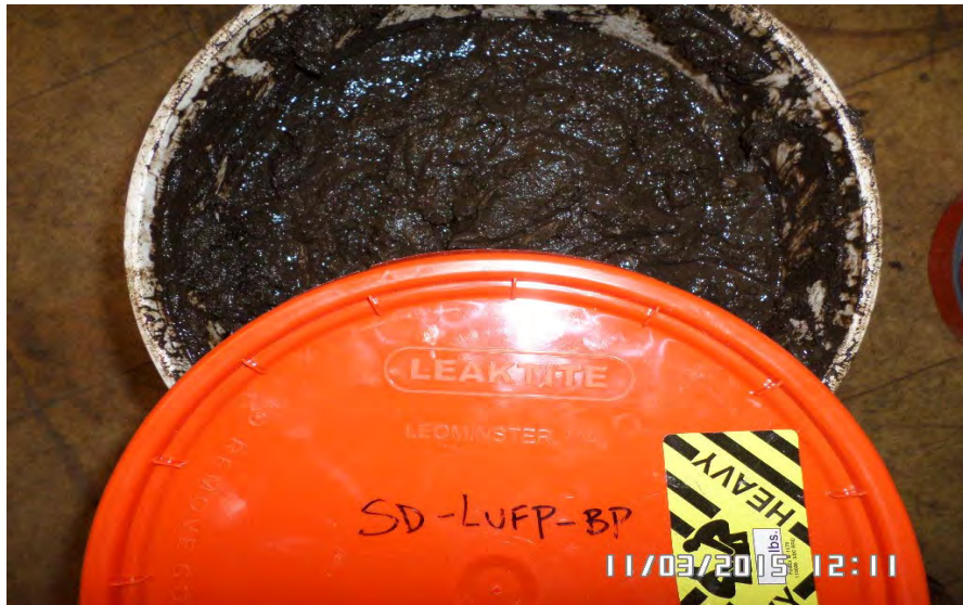
LUFP-BP Sediment after light homogenization.
