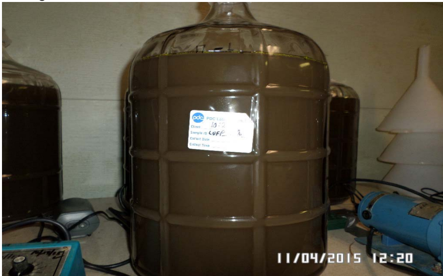
LUFP-BP Sediment Slurry (1 hour aeration at 0.5% solids) after one hour settling.
