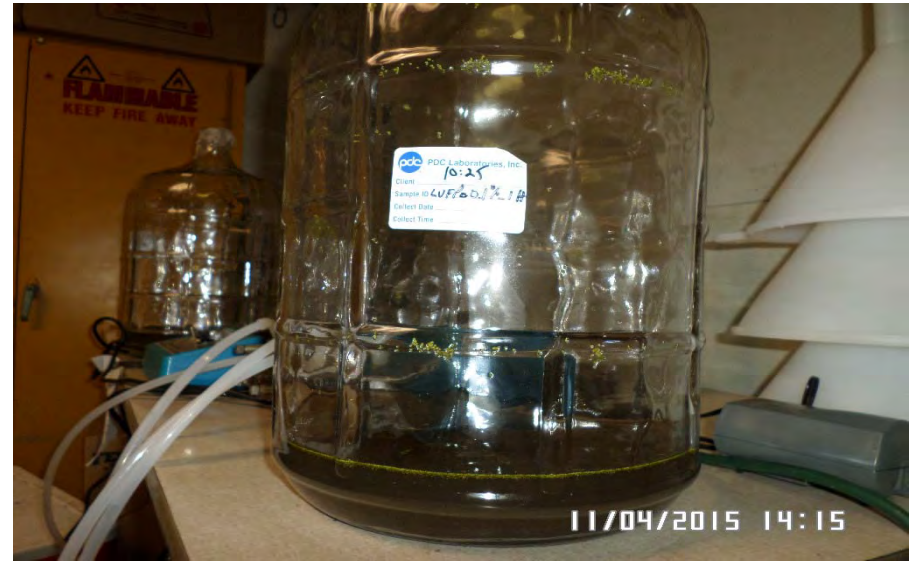
LUF2-BP Sediment after pumping off supernatant (1 hour aeration at 0.1% solids).
