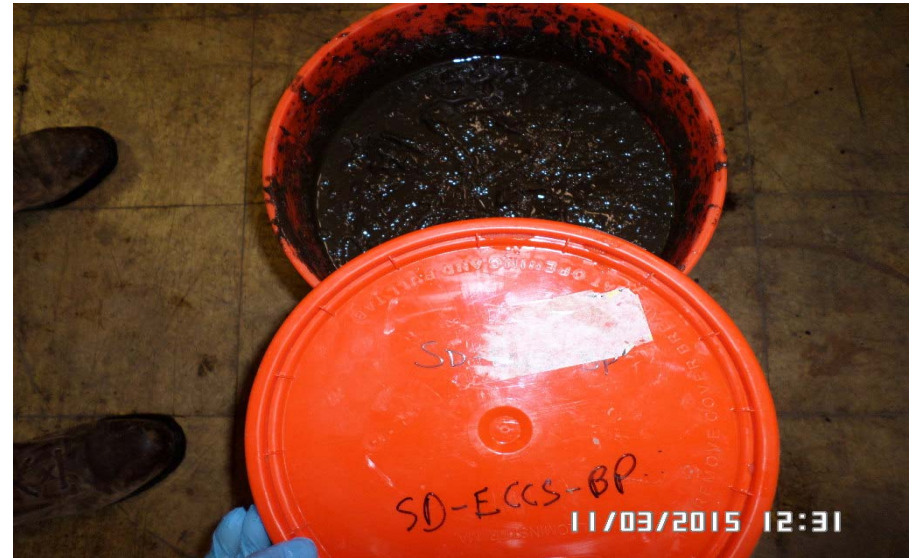
ECCS-BP Sediment after light homogenization.
