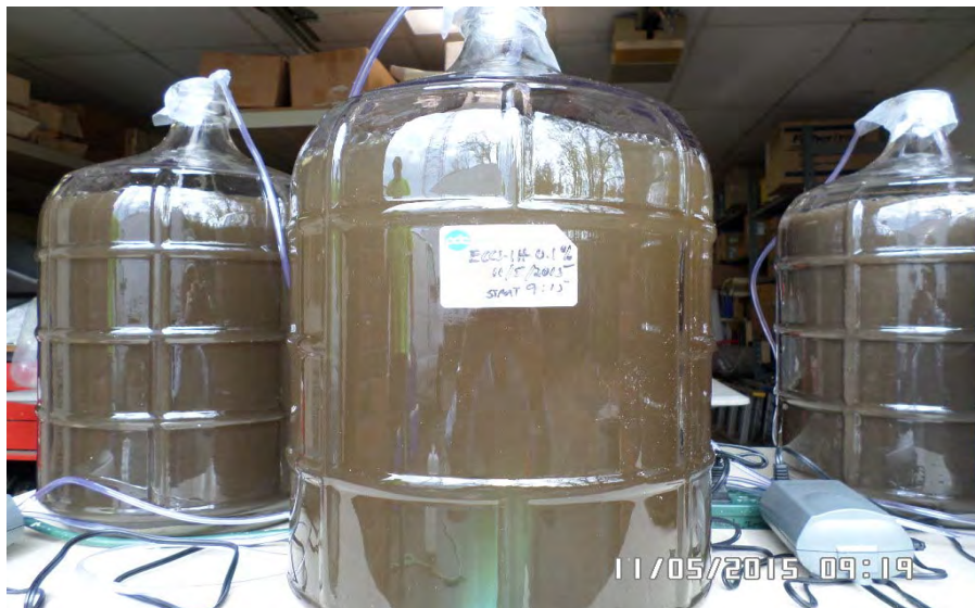
ECCS-BP Sediment Slurry (1 hour aeration at 0.1% solids) during aeration stage.
