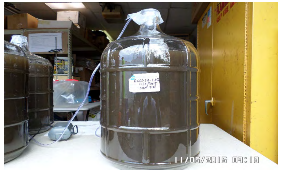
ECCS-BP Sediment Slurry (1 hour aeration at 1.0% solids) during aeration stage.
