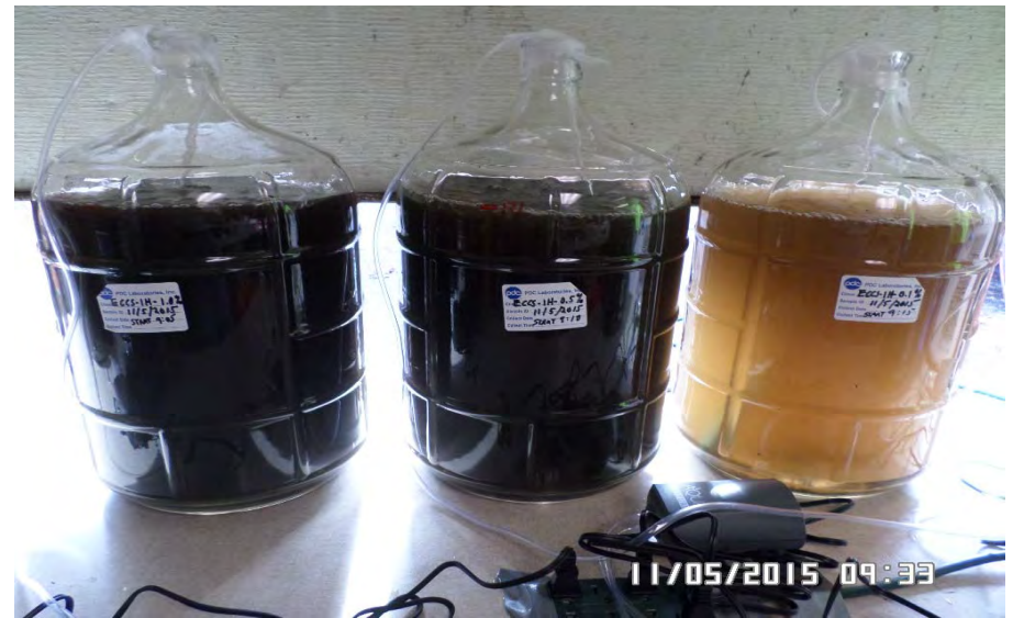
3 ECCS –BP Sediment Slurries (1.0%, 0.5%, and 0.1% solids) during 1 hour aeration stage.
