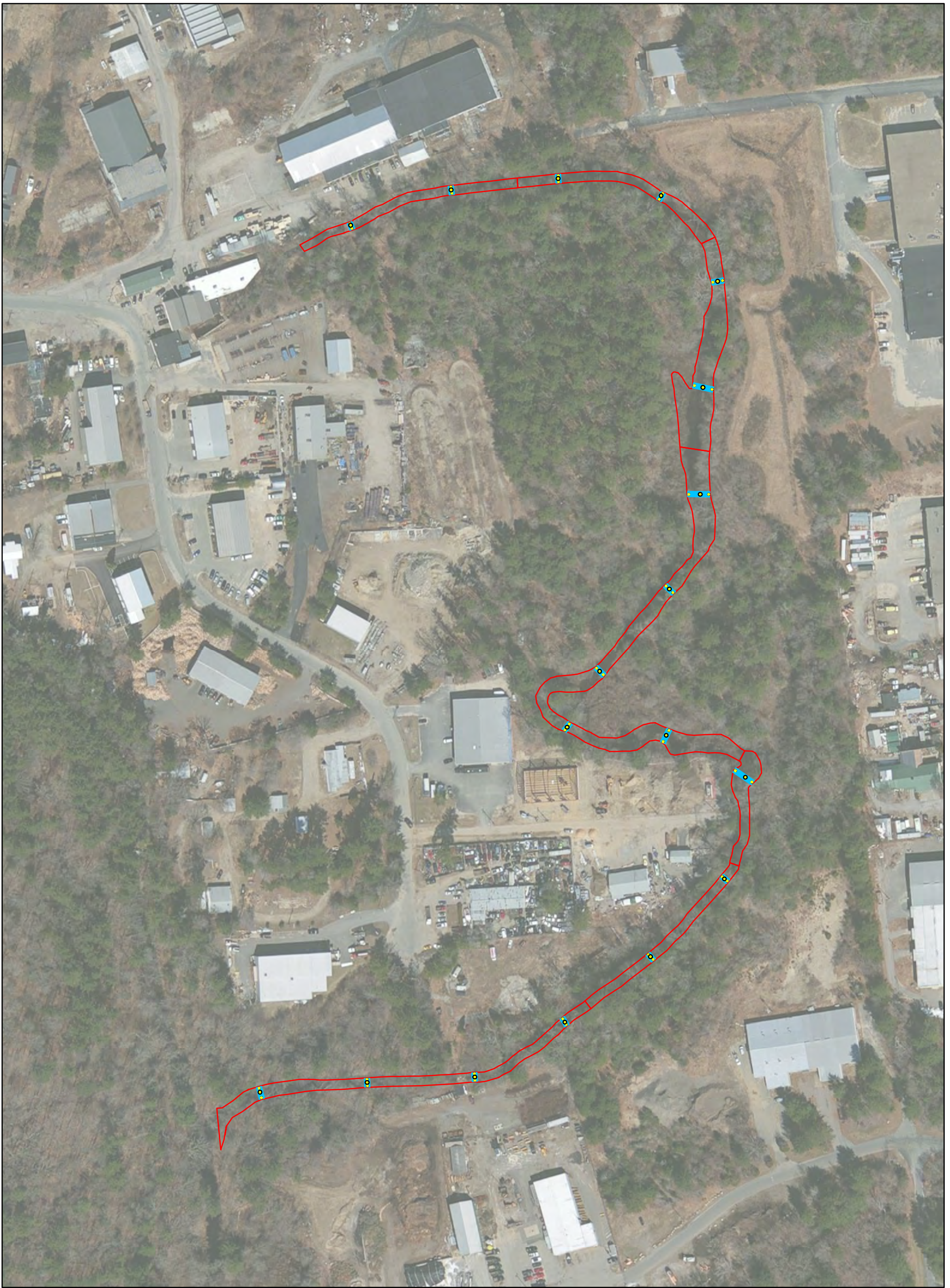
Figure 5: Proposed Eastern Channel Corridor Sediment Sampling Transect Locations
