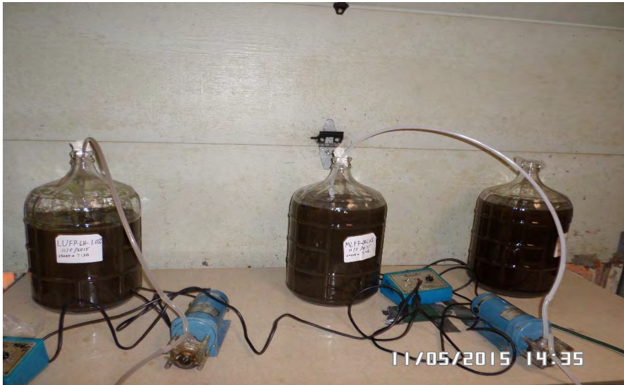
Pumping off 6 hour aeration supernatants (LUFP-BP and MLFP-BP) after one hour settling stage.
