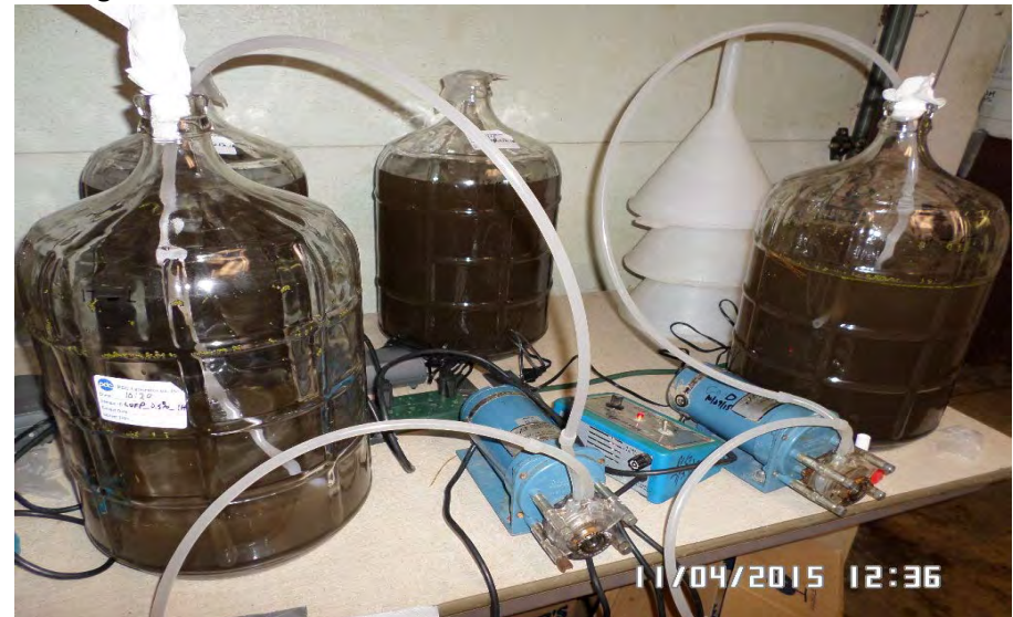
Pumping off LUFP-BP supernatants after one hour settling period. (View 1 of 2)
