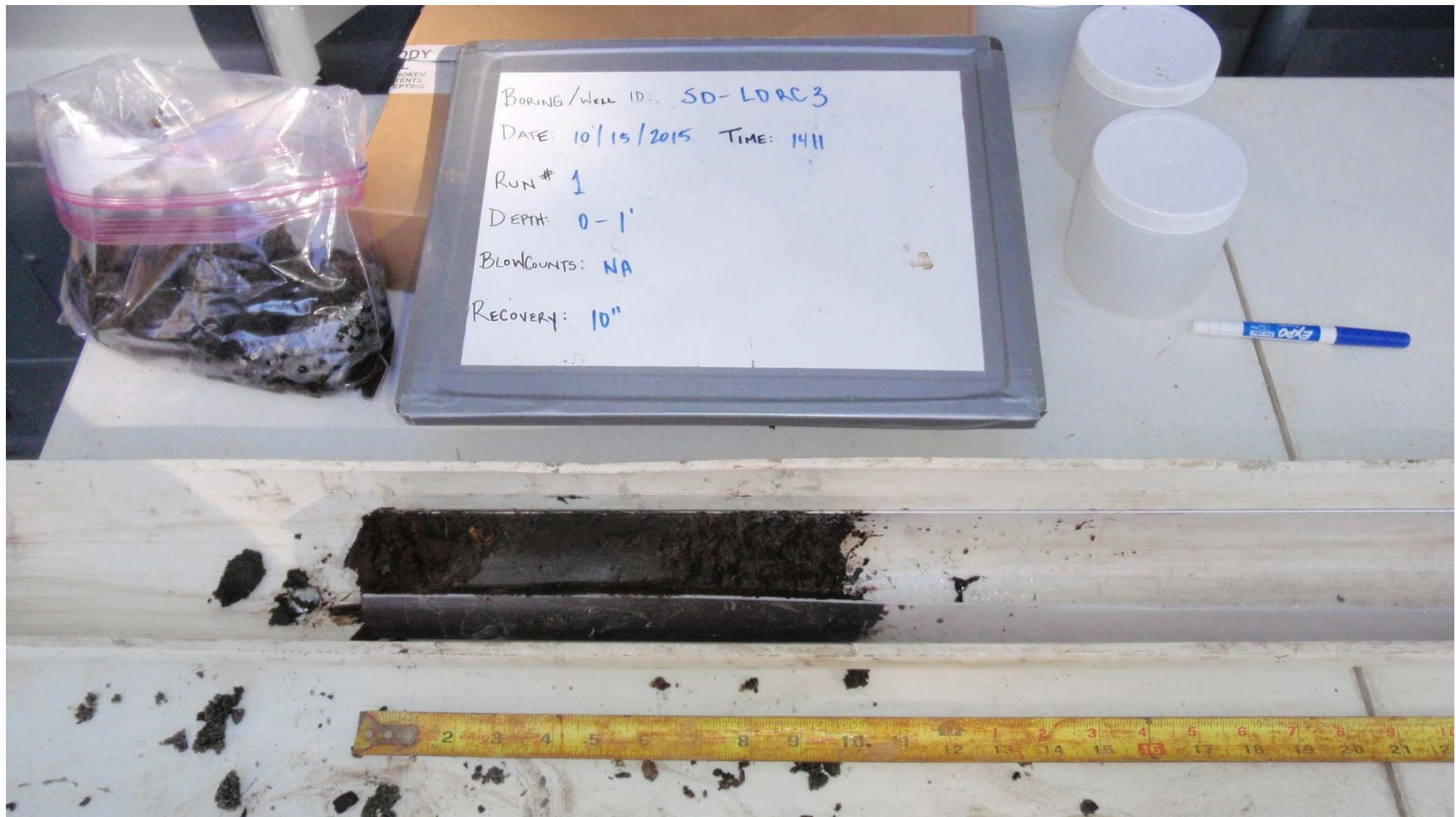
Photo 5-B1. Core of representative sediment from which geotechnical sample SD-LDRC-GT was collected.
