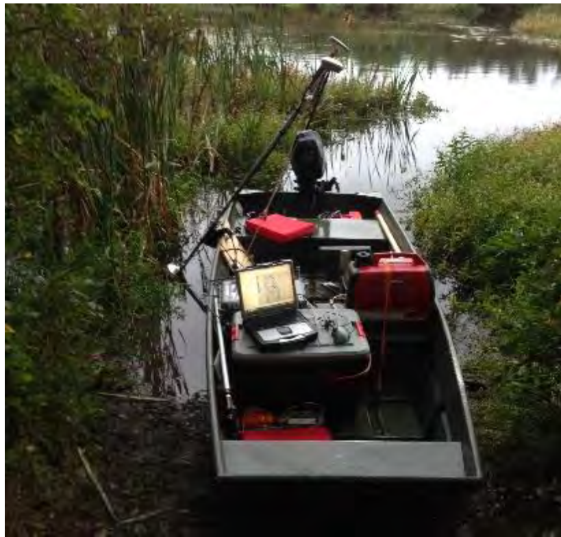
Figure 1. Single Beam Survey Vessel (sonar pole stored on angle, not survey ready)
