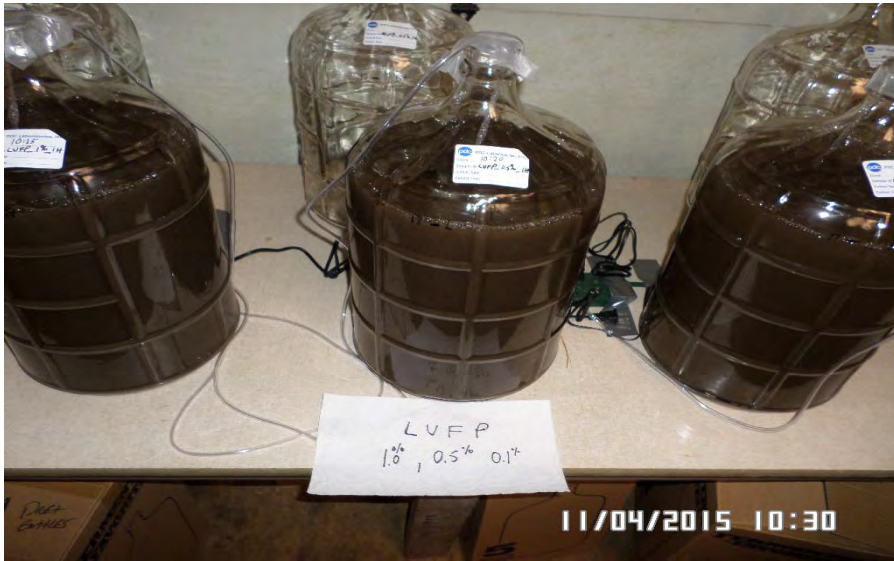
3 LUF BP Sediment Slurries (1.0%, 0.5%, and 0.1% solids).
