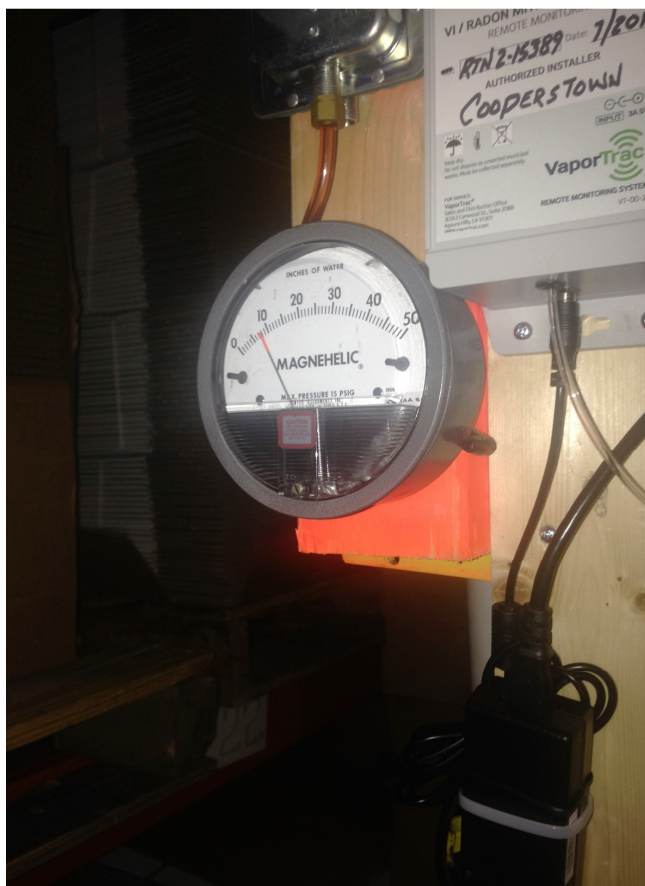
Photograph #2: View of the Magnehelic gauge associated with Telemetry Device #1 at the Site.
